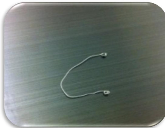
Figure 65: Wire for short-circuiting GPIO_9 to VCCC.
