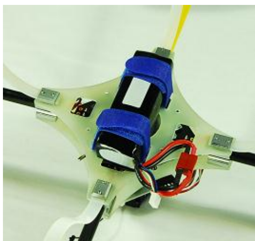
26 Fix the battery below upper cover using the Velcro fastener tightly
