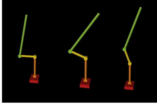
Figure 5.3: The three positions of the system linearization. Every position is a point of linearization and defines a linear system.
