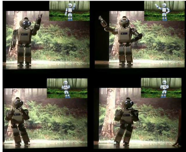
Figure 2.23: Dance performance of the humanoid robot HOAP-3 in the robotics show. In the image it can be seen a synchronized simulation of the dance in OpenHRP simulator.
