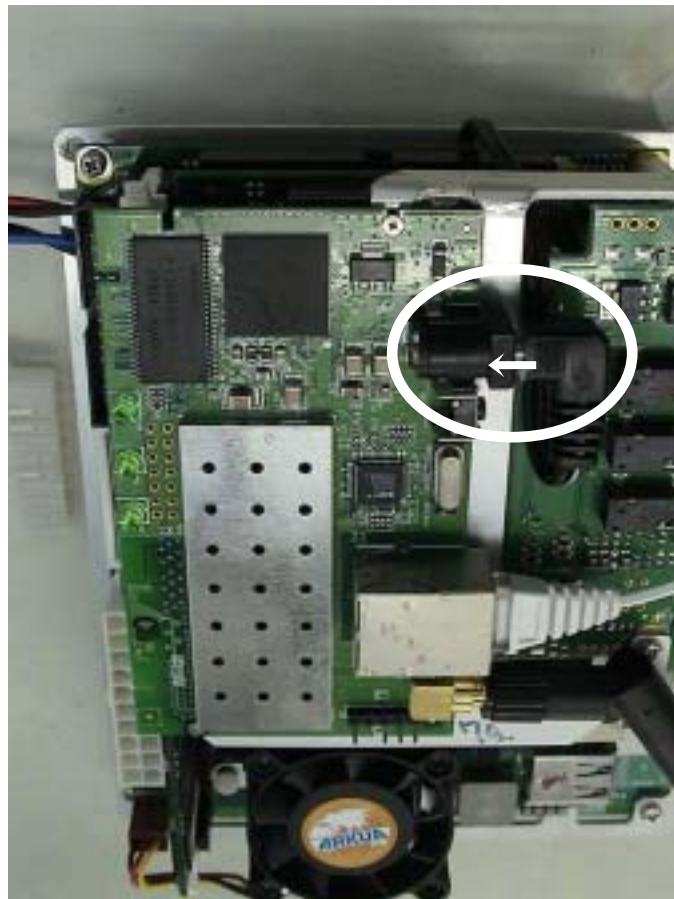
Fig.3.2-3 The power supply line of a wireless LAN converter
