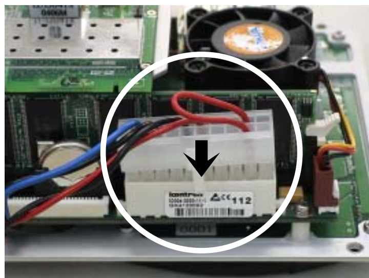
Fig.3.2-4 Power supply of Inside PC
