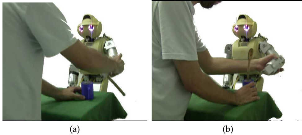
Figure 4.2: Kinaesthetic Teaching of the Skill: (a) Teaching of a spoon in the cup task. (b) Teaching of a grasp task.
