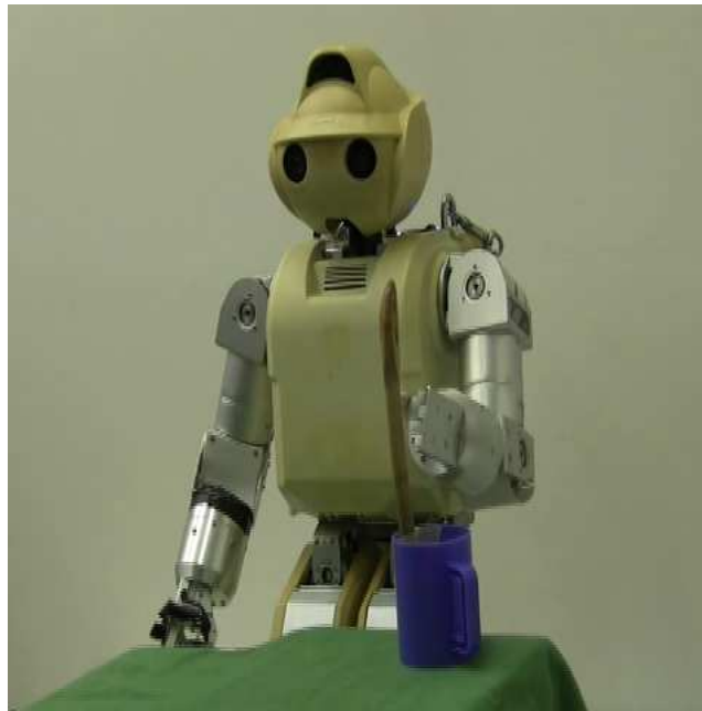
Figure 6.8: The HOAP-3 robot is teach to reproduce a “reach and grasp spoon” task
