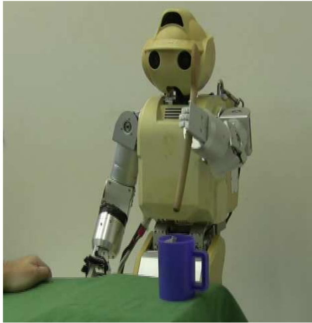
Figure 6.7: The HOAP-3 robot is teach to reproduce a “place spoon in a cup” task
