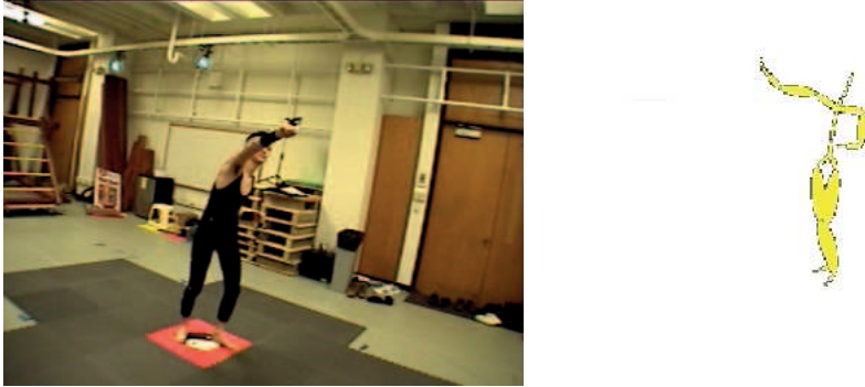
Fig. 3.5: Demonstrations in a Motion Capture Systems: (left) A human teacher performs a demonstration. (right) The generated skeleton of the human recorded demonstration.
